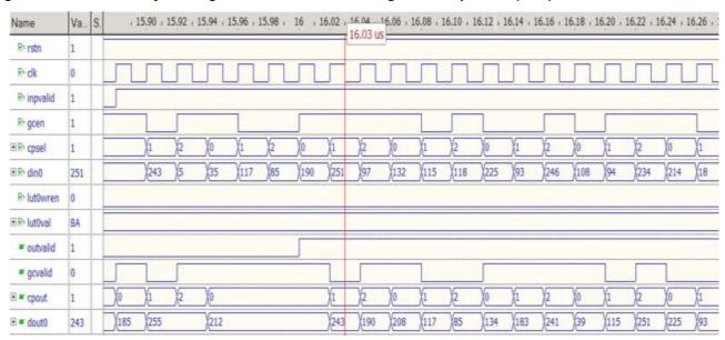
Figure 2-8. Functionality of Constant Gamma Value (= 2.2)
