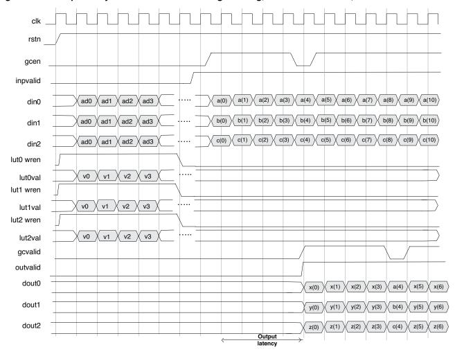
Figure 2-7. Functionality of Programmable Gamma through Look-Up Table (LUT)
