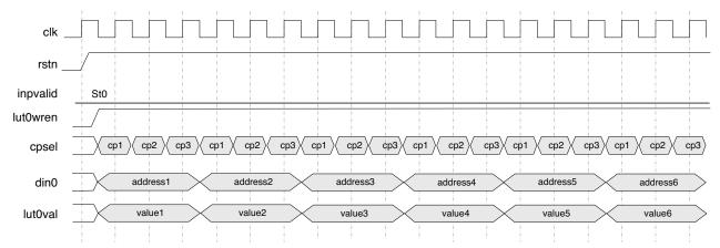
Figure 2-6. Example of Dynamic Gamma Value Programming, Three Color Planes, Parallel Mode
