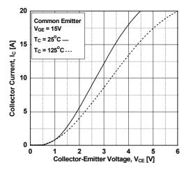
Figure 5. Saturation Voltage vs. Case
