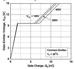
Figure 11. Turn-on Characteristics vs.
