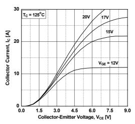
Figure 4. Transfer Characteristics
