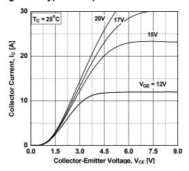
Figure 3. Typical Saturation Voltage Characteristics
