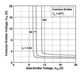
Figure 7. Saturation Voltage vs. V<sub>GE</sub>
