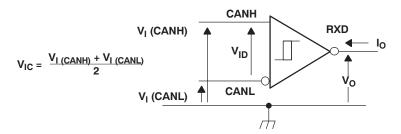
Figure 5. Receiver Voltage and Current Definitions
