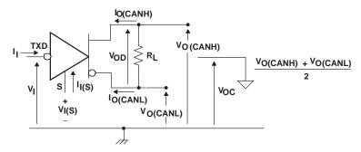
Figure 1. Driver Voltage, Current, and Test Definition
