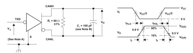
Figure 4. Driver Test Circuit and Voltage Waveforms
