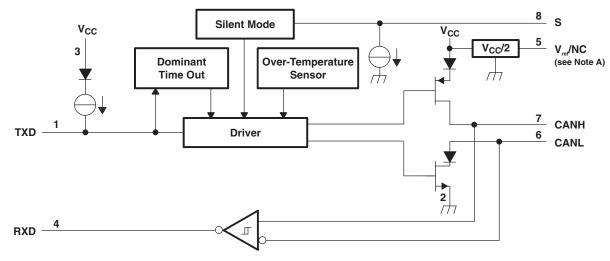
A. V<sub>ref</sub> on SN65HVD1050A, NC on SN65HVD1050AL
