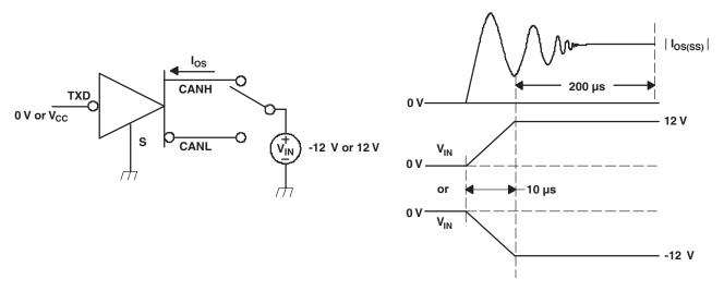
Figure 11. Driver Short-Circuit Current Test and Waveforms
