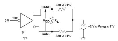
Figure 3. Driver V<sub>OD</sub> Test Circuit
