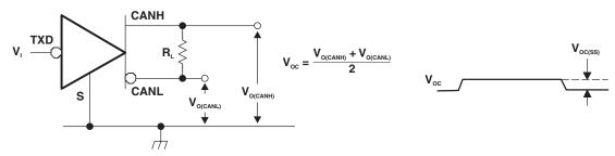
NOTE: All V<sub>I</sub> input pulses are from 0 V to V<sub>CC</sub> and supplied by a generator having the following characteristics:  $t_r$  or  $t_f \le 6$  ns, pulse repetition rate (PRR) = 125 kHz, 50% duty cycle.
