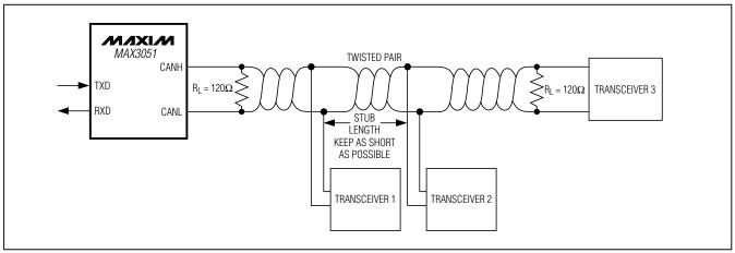
Figure 6. Multiple Receivers Connected to CAN Bus
