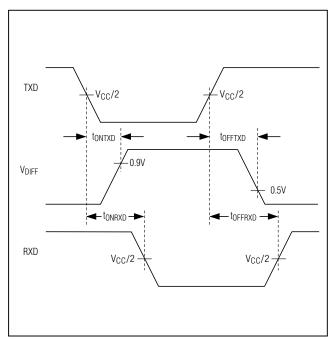
Figure 1. Timing Diagram
