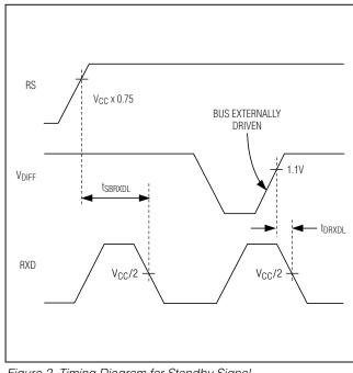
Figure 2. Timing Diagram for Standby Signal
