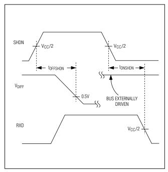
Figure 3. Timing Diagram for Shutdown Signal
