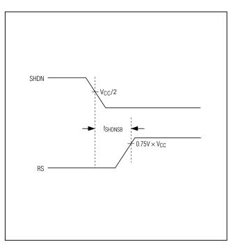
Figure 4. Timing Diagram for Shutdown-to-Standby Signal
