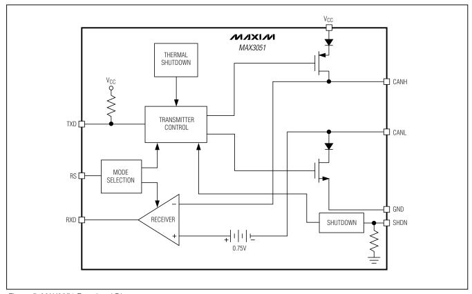
Figure 5. MAX3051 Functional Diagram
