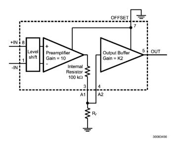
FIGURE 3. Reduce Gain for Unidirectional Application
