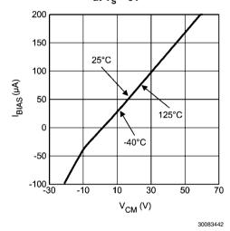
Input Bias Current Over Temperature (A2 pin) at  $V_S = 5V$
