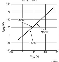
Input Bias Current Over Temperature (+IN and -IN pins) at  $V_S = 5V$
