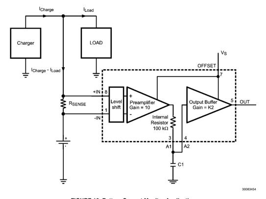
FIGURE 12. Battery Current Monitor Application
