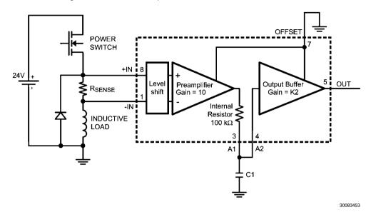
FIGURE 11. High Side Current Sensing Application with Negative Common Mode Transients
