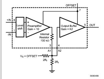
FIGURE 4. Reduce Gain for Bidirectional Application
