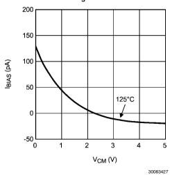
Input Bias Current Over Temperature (A2 pin) at  $V_S = 5V$
