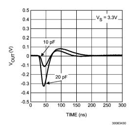
FIGURE 7. Capacitive Load Response at 3.3V
