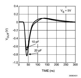
FIGURE 8. Capacitive Load Response at 5.0V
