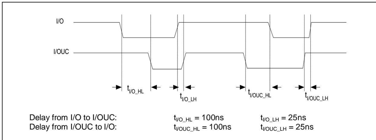
Figure 7: I/O – I/OUC Delays Timing Diagram
