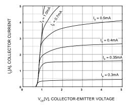
Figure 1. Static Characteristic
