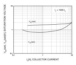
Figure 3. Base-Emitter Saturation Voltage Collector-Emitter Saturation Voltage
