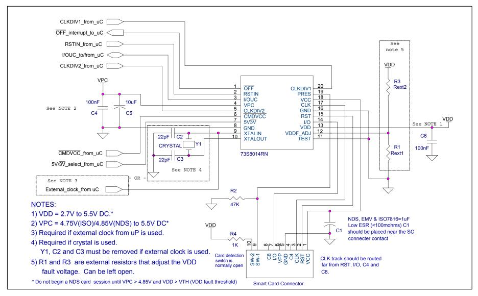
Figure 3: 73S8014RN – Typical Application Schematic
