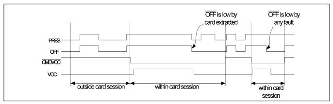
Figure 7: Timing Diagram – Management of the Interrupt Line OFF
