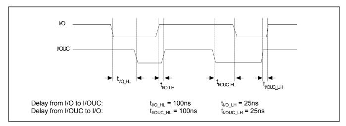
Figure 9: I/O – I/OUC Delays – Timing Diagram
