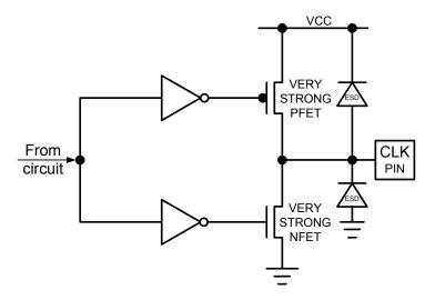
Figure 12: Type 5 – Smart Card CLK Driver Circuit
