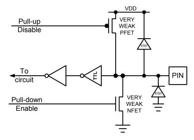
Note: Pins  $\overline{\text{CMDVCC}}$ , 5V/ $\overline{\text{3V}}$ , CLKDIV1 and CLKDIV2 have the pull-up enabled. Pins RSTIN, CLKIN, PRES have the pull-down enabled.
