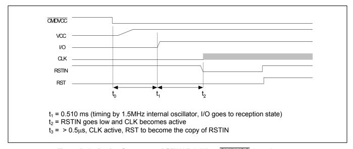
Figure 5: Activation Sequence – RSTIN High When CMDVCC Goes Low
