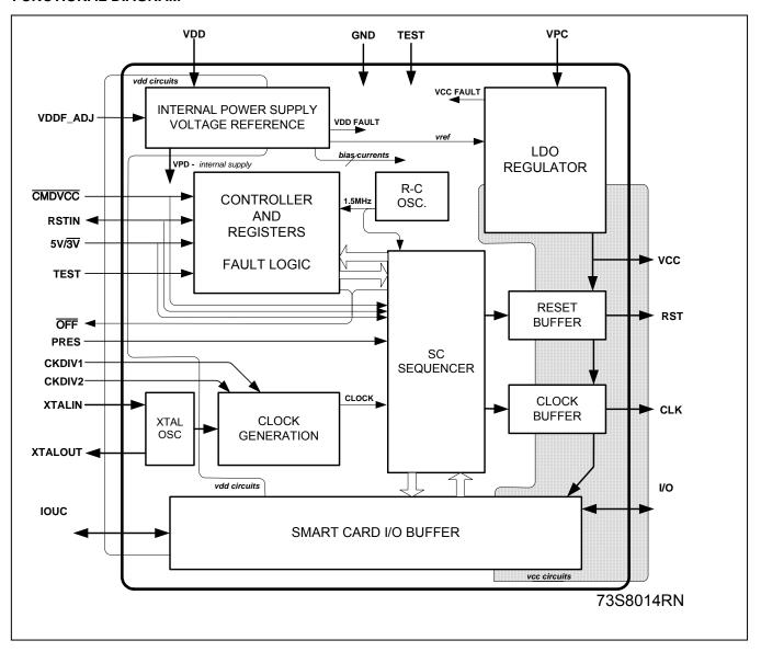
Figure 1: 73S8014RN Block Diagram
