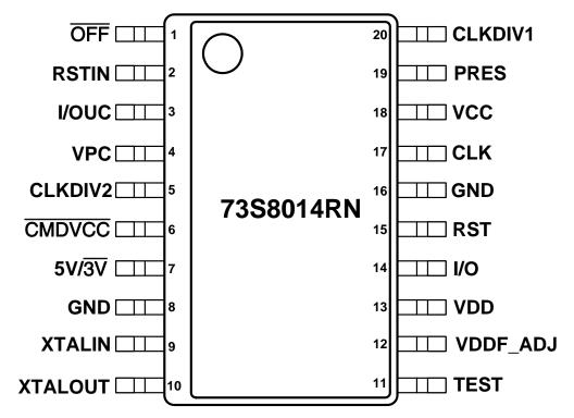
Figure 2: 73S8014RN 20-SOP Pin Out
