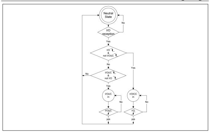
Figure 8: I/O and I/OUC State Diagram
