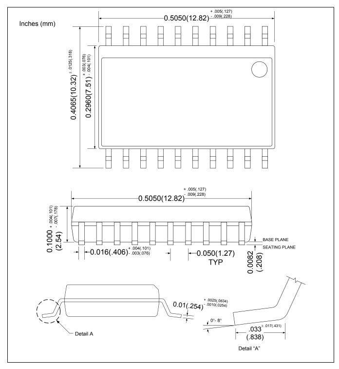
Figure 19: Mechanical Drawing 20-Pin SO Package
