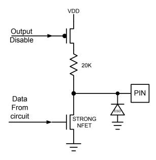
Figure 10: Open Drain type – OFF
