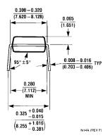
Molded Dual-In-Line Package (N) Order Number LM361N NS Package Number N14A
