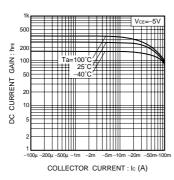
Fig.3 DC current gain vs. collector current
