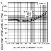
Fig.2 Collector-emitter saturation voltage vs. collector current
