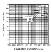
Fig.1 DC current gain vs. collector current
