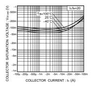
Fig.4 Collector-emitter saturation voltage vs. collector current
