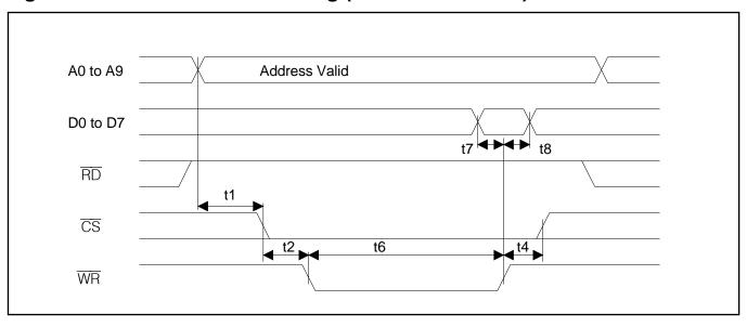
Figure 38-6. Motorola Bus Read Timing (BTS = 1 / MUX = 0)
