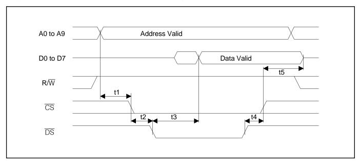
Figure 38-7. Motorola Bus Write Timing (BTS = 1 / MUX = 0)
