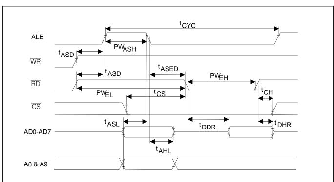
Figure 38-1. Intel Bus Read Timing (BTS = 0 / MUX = 1)
