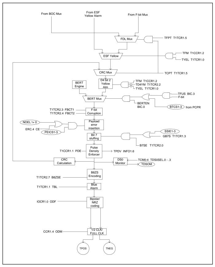
Figure 34-3. E1 Transmit Data Flow
