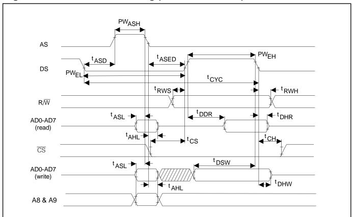
Figure 38-3. Motorola Bus Timing (BTS = 1 / MUX = 1)
