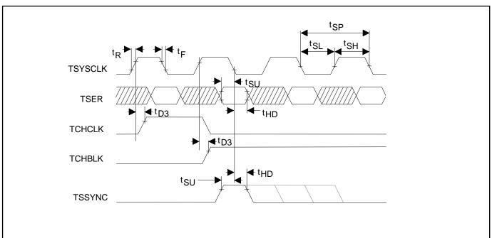
Figure 38-14. Transmit Side Timing, Elastic Store Enabled
