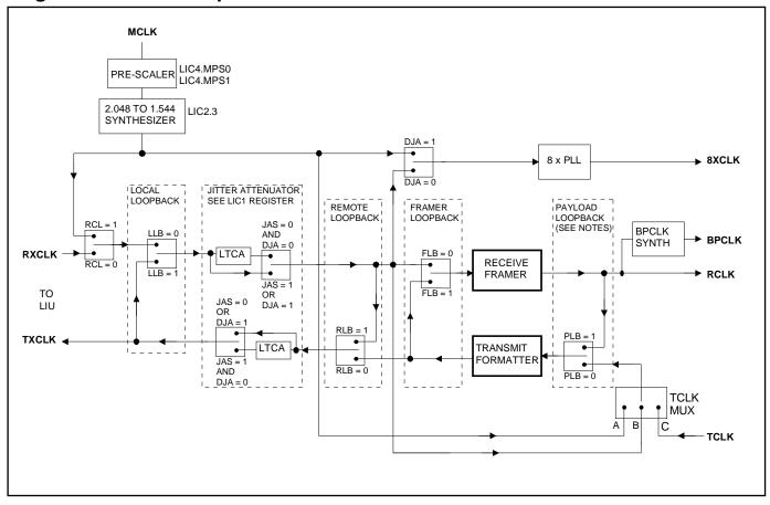
The TCLK MUX is dependent on the state of the TCSS0 and TCSS1 bits in the LIC1 register and the state of the TCLK pin.
