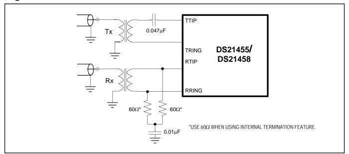
Figure 25-2. Basic Unbalanced Network Connections
