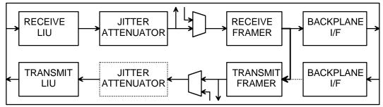
PAYLOAD LOOPBACK (CAN BE DONE ON A PER-CHANNEL BASIS)
