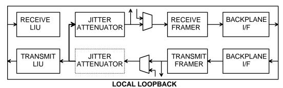
**Bit 4/Line Interface Unit Mux Control (LIUC).** This bit along with the LIUC/TPD pin and LBCR.7 controls the connection between the LIU and the Framer. See the LTS (LBCR.7) description below. When the LIUC/TPD pin is connected high or LBCR.7 = 1, the LIUC bit has control. When the LIUC/TPD pin is connected low the framer and LIU are separated and the LIUC bit has no effect. For the DS21458 this bit should always be set = 0.
