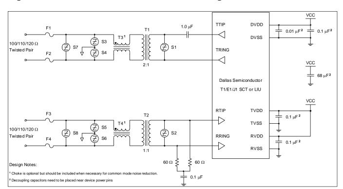
Figure 25-6. Software-Selected Termination, Longitudinal Protection
