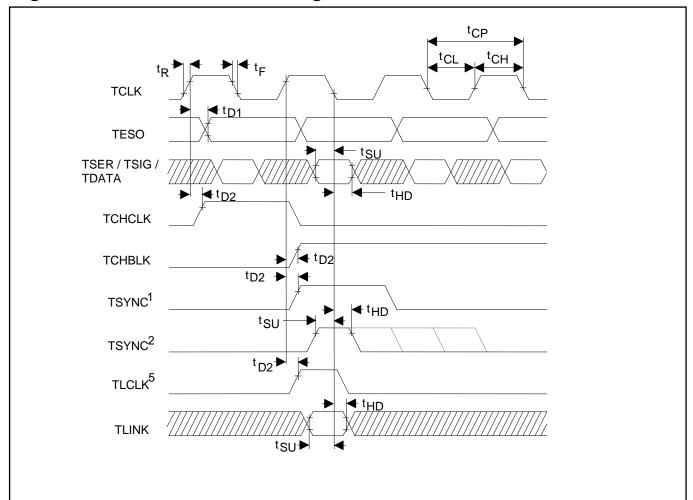
Figure 38-13. Transmit Side Timing
