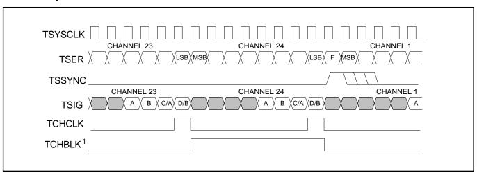
1) TCHBLK is programmed to block channel 24 (if the TPCSI bit is set, then the signaling data at TSIG will be ignored during channel 24).
