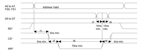
Figure 23-6. MOTOROLA BUS READ AC TIMING (BTS = 1 / MUX = 0)
