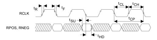
Figure 23-11. TRANSMIT SIDE AC TIMING
