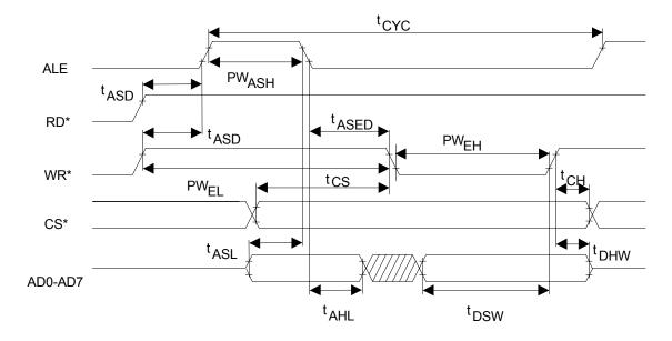
Figure 23-3. MOTOROLA BUS AC TIMING (BTS = 1 / MUX = 1)
