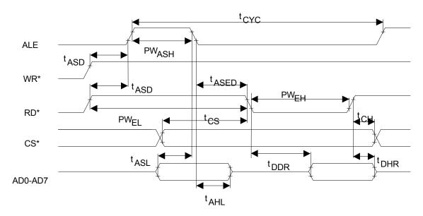
Figure 23-2. INTEL BUS WRITE TIMING (BTS = 0 / MUX = 1)
