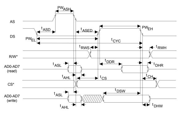
Figure 23-4. INTEL BUS READ AC TIMING (BTS = 0 / MUX = 0)
