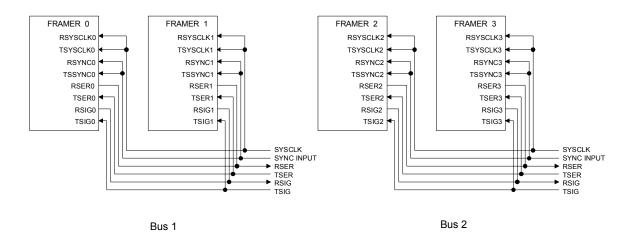
Figure 20-2. 8.192MHz INTERLEAVED BUS EXTERNAL PIN CONNECTION EXAMPLE
