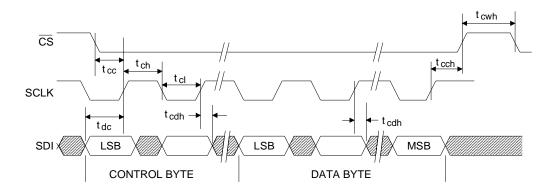
Figure 4. Serial Port Write Timing Diagram
