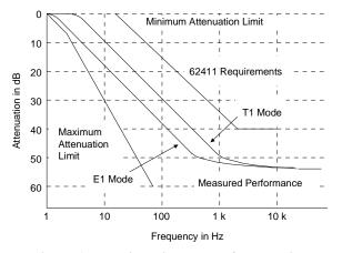
Figure 17. Typical Jitter Transfer Function
