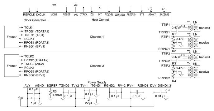
Figure 29. Host Mode Parallel Port Configuration
