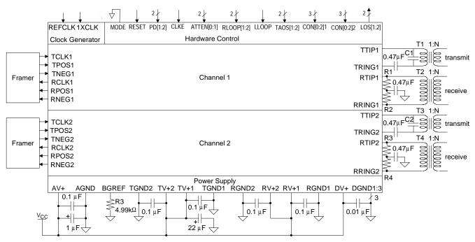
Figure 27. Hardware Mode Configuration
