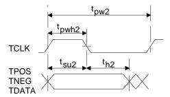
Figure 3. Transmit Clock and Data Switching Characteristics
