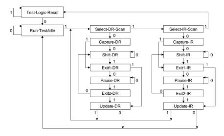
Figure 24. TAP Controller State Diagram
