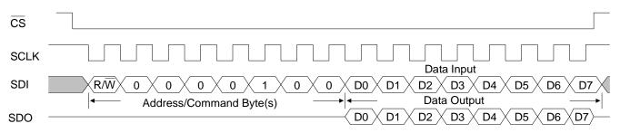
Figure 21. Serial Read/Write Format (SPOL = 0)
