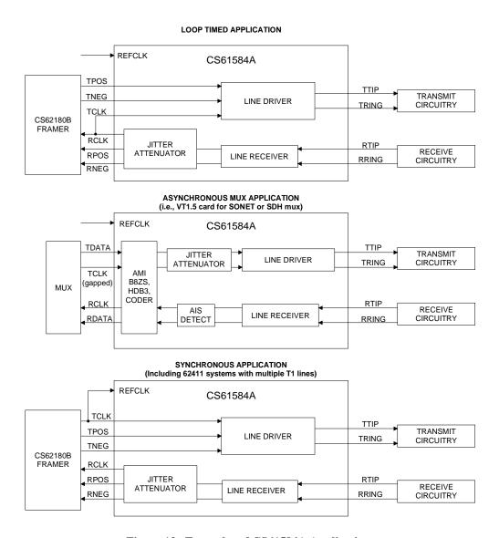
Figure 13. Examples of CS61584A Applications
