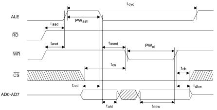
Figure 8. Parallel Port Timing - Intel Write Mode
