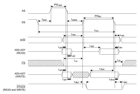
Figure 6. Parallel Port Timing - Motorola Mode
