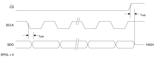
Figure 5. Serial Port Read Timing Diagram
