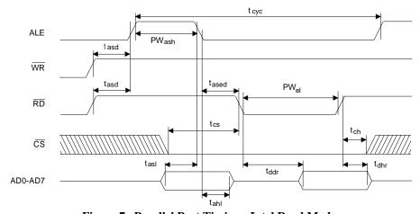
Figure 7. Parallel Port Timing - Intel Read Mode
