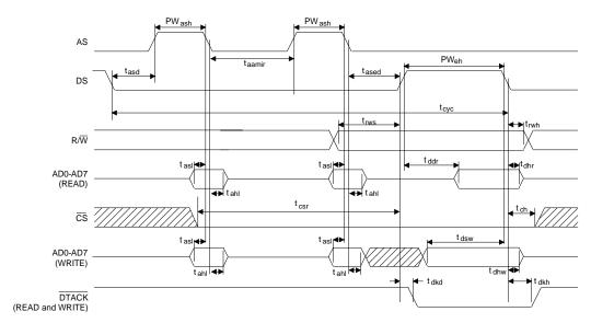
Figure 9. Parallel Port Timing - Motorola Mode to RAM
