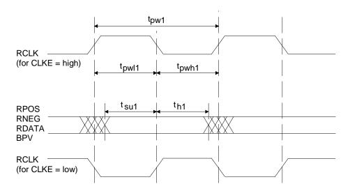
Figure 2. Recovered Clock and Data Switching Characteristics
