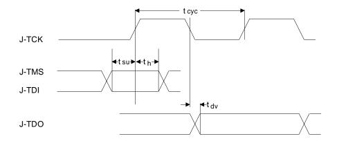
Figure 12. JTAG Switching Characteristics
