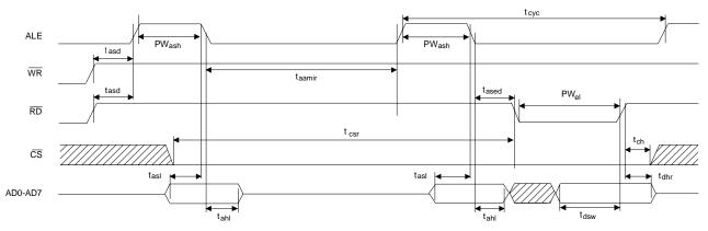
Figure 11. Parallel Port Timing - Intel Write Mode to RAM
