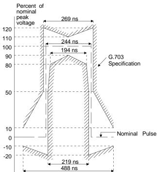
Figure 14. Typical Pulse Shape at DSX-1 Cross Connect
