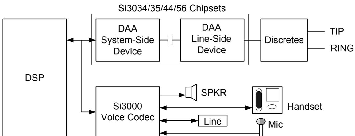
Figure 14. Si3000 with Silicon Labs DAA System Diagram
