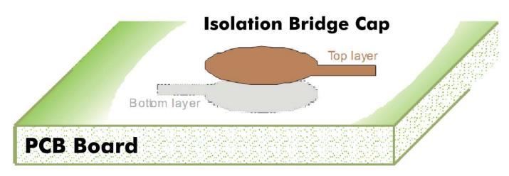
The application requires three PCB capacitors whose diameters range typically from 140 to 190 mils depending on the thickness of the board.
