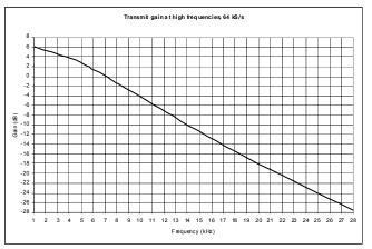
Figure 4. Transmit Gain at High Frequencies (600  $\Omega$ )
