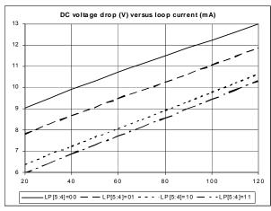
Figure 10. DC Voltage vs. Current, No Regulation
