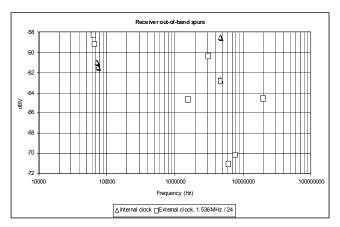
Figure 25. Receiver Out-of-Band Spurs
