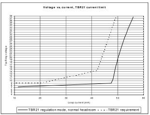
Figure 13. DC Voltage vs. Current, TBR21 Regulation
