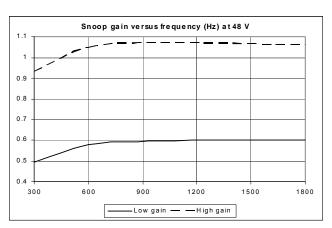
Figure 8. Snoop Gain versus Frequency
