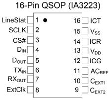
Figure 34. Pin Configuration
