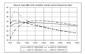
Figure 11. Return Loss for Resistive Modes
