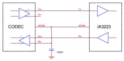
Figure 33. Differential Interface (With Reference)
