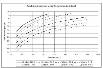
Figure 17. Parallel Pickup Sensitivity to Transmitted Signals
