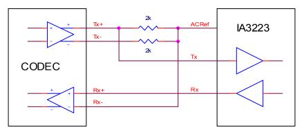
Figure 32. Differential interface (Without Reference)
