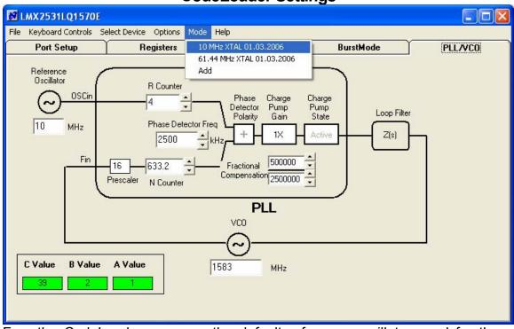
For the CodeLoader program, the default reference oscillator used for these instructions was 10 MHz, but there is a mode for a 61.44 MHz oscillator as well. If the bits become scrambled, their original state may be recalled by choosing the appropriate mode. Note that if the internal divide by 2 is enabled, the VCO frequency still reflects the VCO frequency before the divide by 2.
