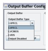
Figure 6. Output Buffer Configuration (each output)
