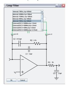
Figure 5. Loop Filter, Internal Only
