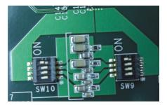
Figure 8. External Loop Filter selection switches
