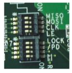
Figure 9. Control Bus ON/OFF Dip Switches
