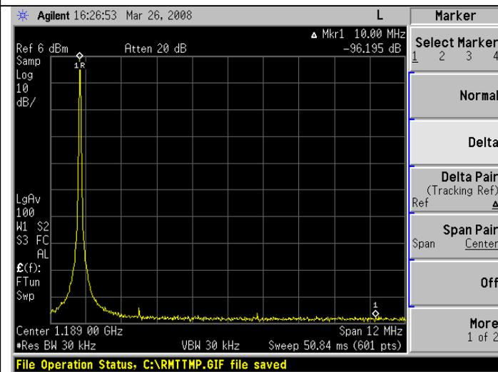
Spur at 10 MHz offset for a frequency of 1184 MHz is below the spectrum analyzer noise floor.
