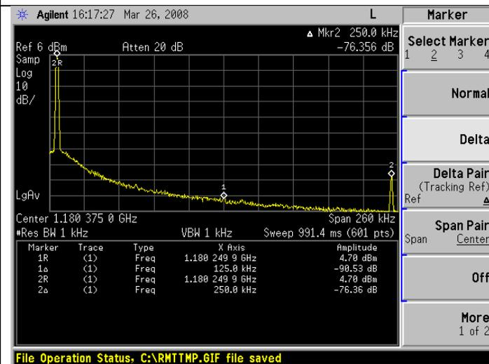
Fractional Spur at 250 kHz offset at a worst case frequency of 1180.25 MHz is -76.4 dBc.
