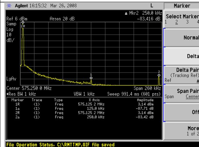
Spur at 250 kHz offset for a frequency of 575.125 MHz is  $-83.4$  dBc.
