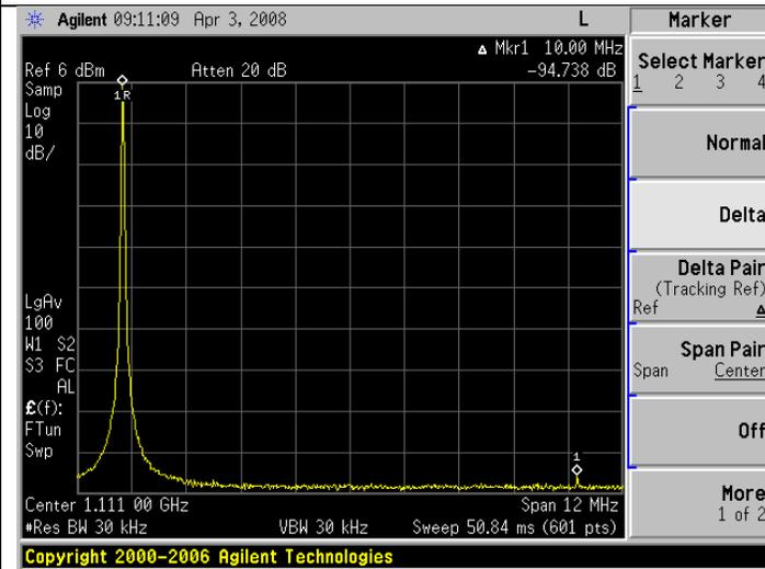
Spur at 10 MHz offset for a frequency of 1106 MHz is -94.7 dBc .
