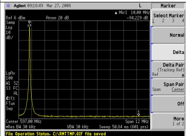
Spur at 10 MHz offset for a frequency of 592 MHz is below the spectrum analyzer noise floor.
