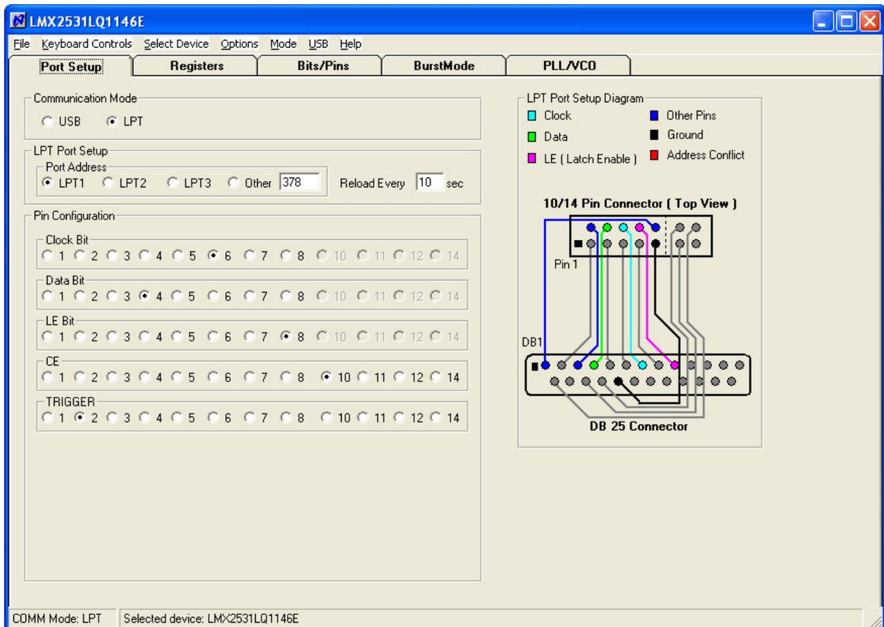
The port setup tells CodeLoader what information goes where. If this is wrong, the part will not program. Although LPT1 is usually correct, CodeLoader does NOT automatically detect the correct port. On some laptops, it may be LPT3.
