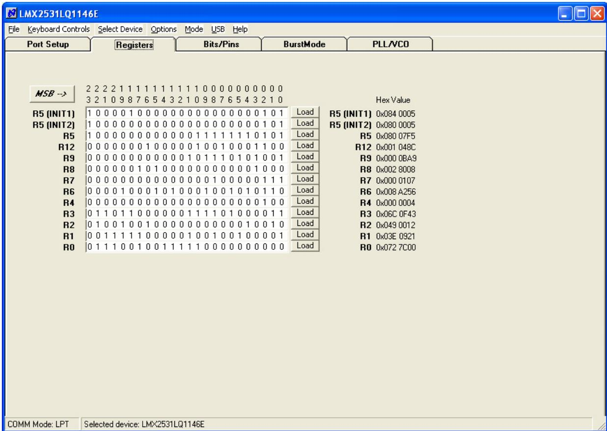
The Registers tab shows the literal bits that are being sent to the part. These are the registers every time the PLL is loaded by using the menu command or Ctrl+L. R5 (INIT1) and R5 (INIT 2) are just the R5 register being used to properly initialize the part. So a single CNT+L will load the part.
