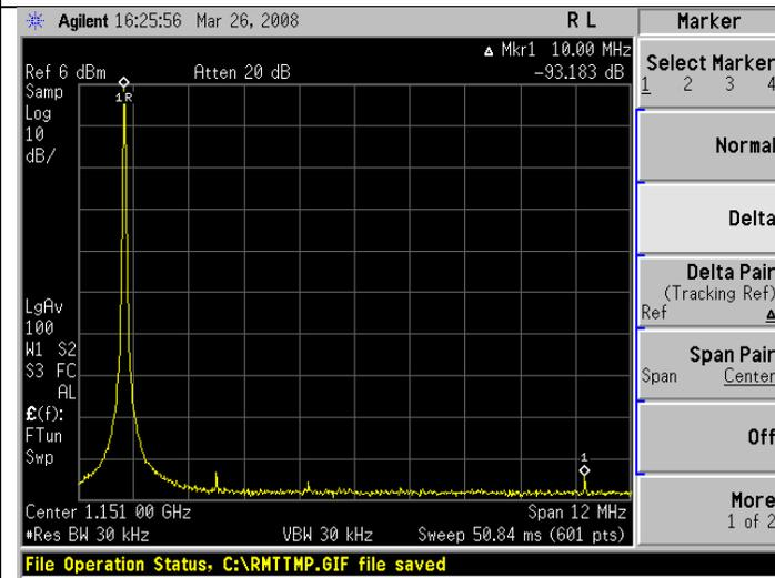
Spur at 10 MHz offset for a frequency of 1146 MHz is -93.2 dBc..
