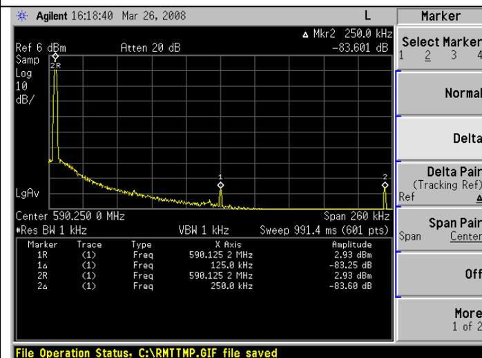
Spur at 250 kHz offset for a frequency of 590.125 MHz is  $-83.6$  dBc.
