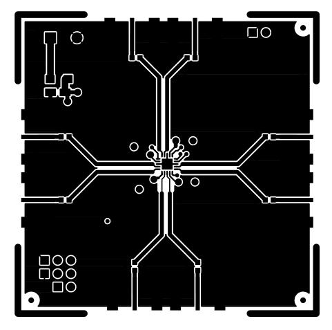
Figure 5. Si5310 Component Side
