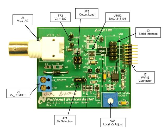
**Figure 1: Component and Test Point Locations**
