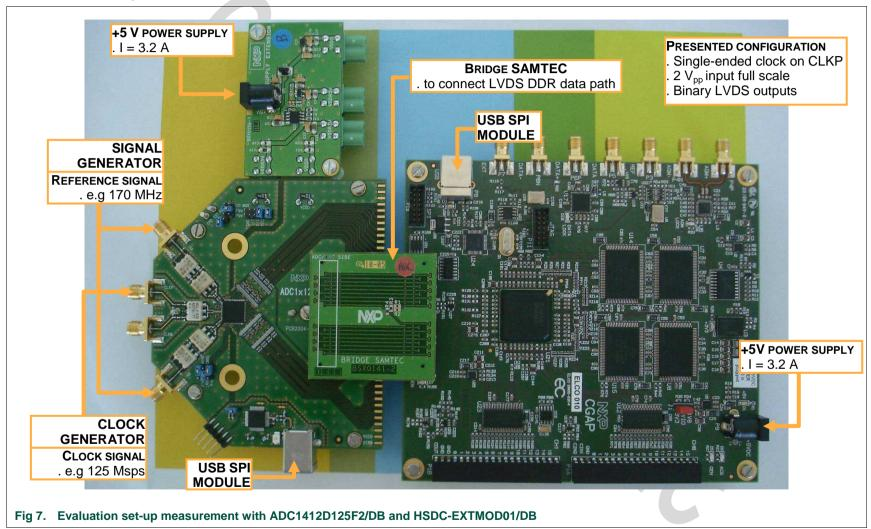
Note 1: make sure that supply extension release B is used: it delivers the 3 V supply for LVDS output path for the ADC.
