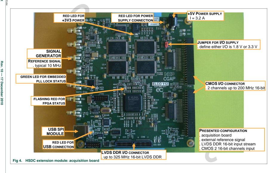
The HSDC extension module is intended for acquisition/generation and clock generation purpose. When connected to an ADC demo-board it is intended as an acquisition system for digital output bits delivered by ADC, either CMOS (HE14 P1 connector) or LVDS DDR (SAMTEC QTH 060 02 P2 connector).
