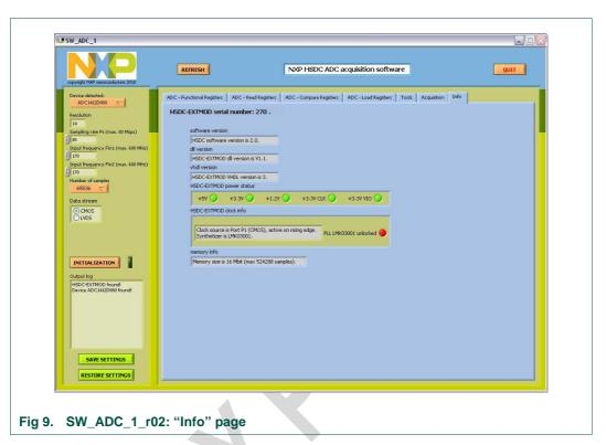
The HSDC-EXTMOD is not yet initialized, so the embedded PLL (LMK03001 in this example) is not locked. Initialization is only required for acquisition purpose.
