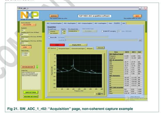
The numbers given for SNR, SFDR are completely wrong if coherency is not respected.
