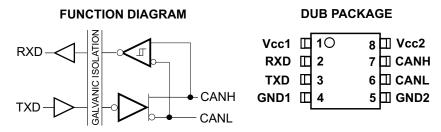
Figure 1. The ISO1050 Function Diagram and Pinout
