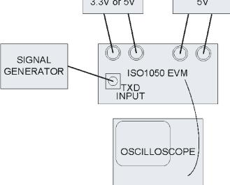
Figure 4. Basic Isolated CAN Transceiver EVM Operation
