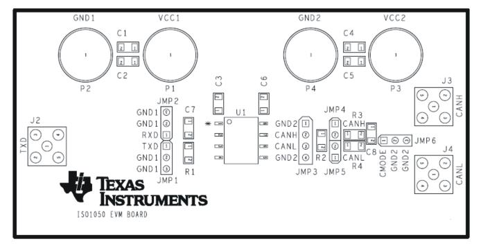
Figure 2. ISO CAN Transceiver EVM Layout
