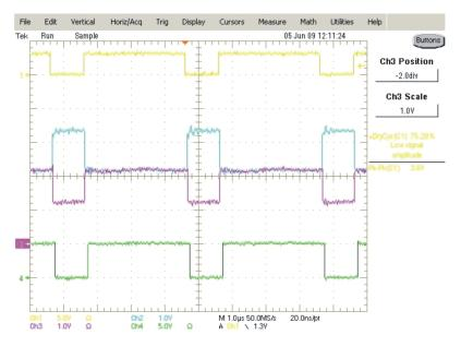
Figure 5. Typical Waveforms Without Common-mode Loading
