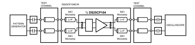
Figure 7. Pre-emphasis and Equalization Performance Test Circuit
