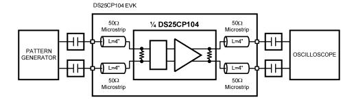
Figure 4. Jitter Performance Test Circuit
