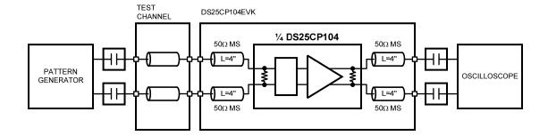
Figure 6. Equalization Performance Test Circuit
