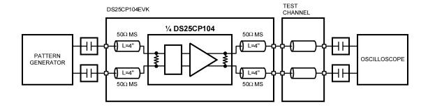
Figure 5. Pre-Emphasis Performance Test Circuit
