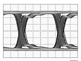
Figure 7. Equalized Signal (40 in FR4, 3.2Gbps, PRBS 7, 0x07 Setting)
