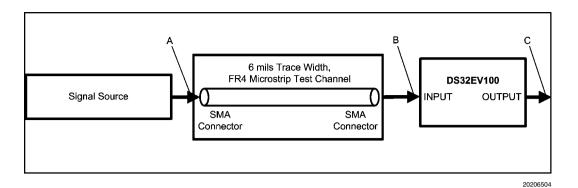
FIGURE 1. Test Setup Diagram
