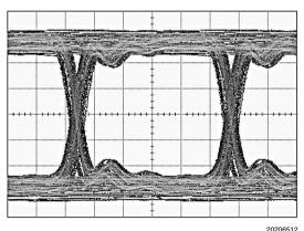
Figure 9. Equalized Signal (32 in Tyco XAUI Backplane, 3.125 Gbps, PRBS 7, 0x07 Setting
