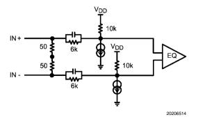
FIGURE 4. Simplified Receiver Input Termination Circuit
