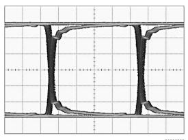
Figure 5. Equalized Signal (40 in FR4, 1 Gbps, PRBS 7, 0x07 Setting)
