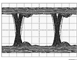
Figure 8. Equalized Signal (10m 24 AWG Twin-AX Cable, 3.2 Gbps, PRBS 7, 0x07 Setting)
