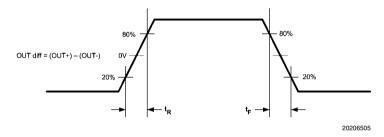
**FIGURE 2. CML Output Transition Times**
