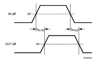
FIGURE 3. Propagation Delay Timing Diagram
