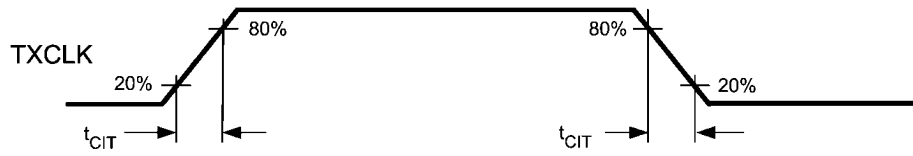
FIGURE 2. Serializer Input Clock Transition Time
