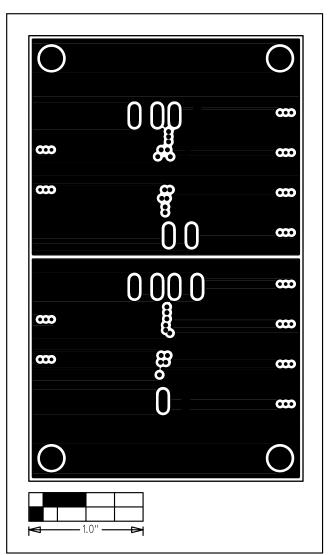
Figure 6. MAX9360 EV Kit PC Board Layout—Inner Layer 3 (VCC Layer)
