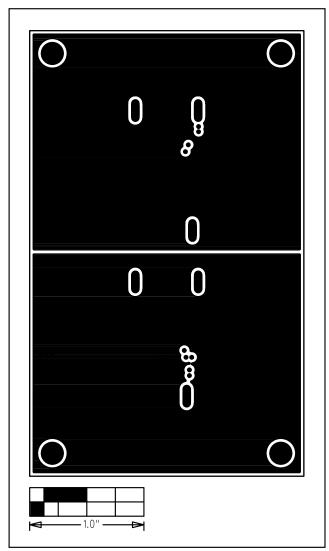
Figure 5. MAX9360 EV Kit PC Board Layout—Inner Layer 2 (Ground Layer)
