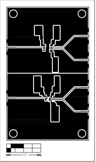
Figure 4. MAX9360 EV Kit PC Board Layout—Component Side
