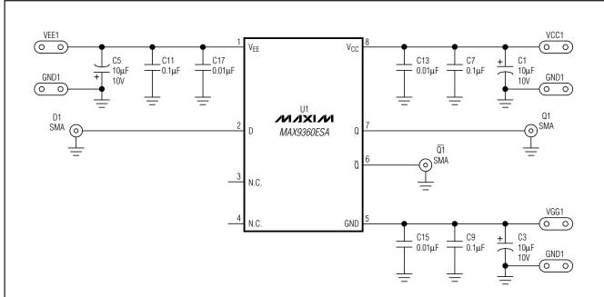
Figure 1. MAX9360 EV Kit Schematic (MAX9360ESA Circuit)
