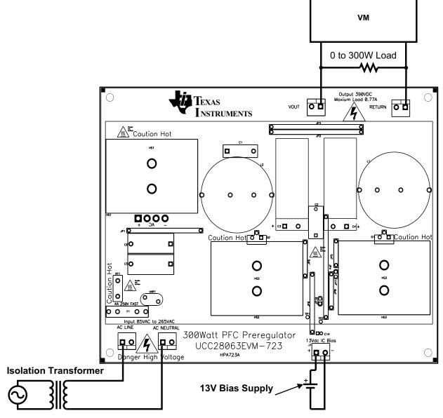
Figure 3. Test Setup
