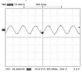
Figure 8. V<sub>out</sub> Ripple, P<sub>out</sub> = 300 W
