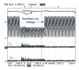
Figure 19. Line Transient, P<sub>OUT</sub> = 300W
