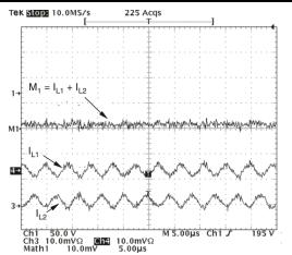
Figure 12. Inductor and Input Ripple Current at 265 V<sub>RMS</sub> Input at Half Peak Line Voltage
