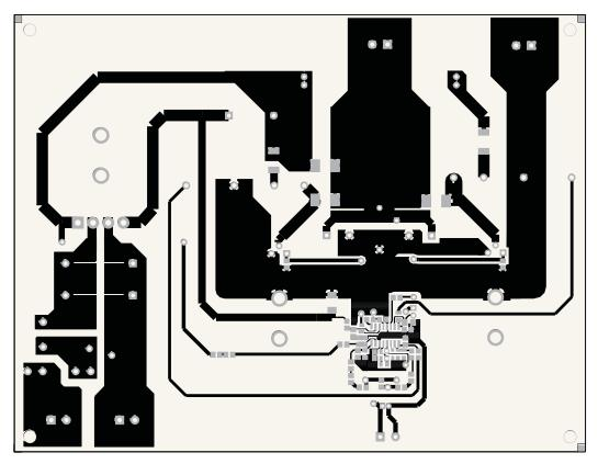
Figure 21. Bottom Layer Copper
