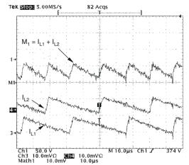
Figure 11. Inductor and Input Ripple Current at 265 V<sub>RMS</sub> Input at Peak Line Voltage
