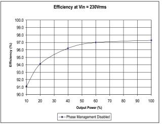
Figure 6. Efficiency at 230  $V_{\text{RMS}}$ , Without Phase Management
