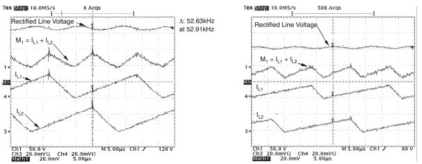
Figure 9. Inductor and Input Ripple Current at 85 V<sub>RMS</sub> Figure 10. Inductor and Input Ripple Current at 85 V<sub>RMS</sub> at Peak of Line Voltage
