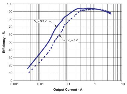
Figure 2. TPS54478EVM-037 Low Current Efficiency
