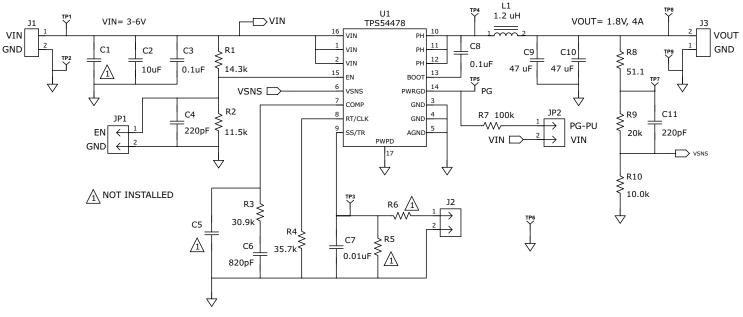
Figure 21. TPS54478EVM-037 Schematic
