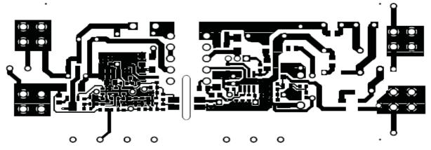
Figure 18. Bottom Copper (bottom view)
