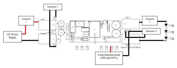
Figure 2. Recommended Test Setup
