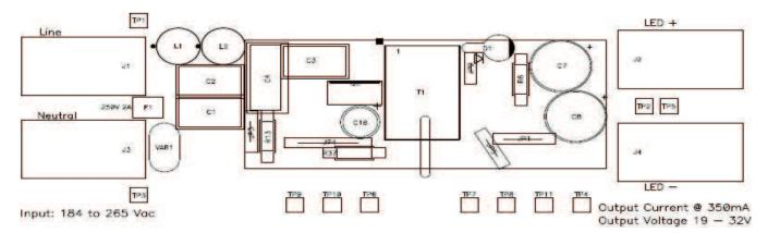
Figure 16. Top Layer Assembly Drawing (top view)
