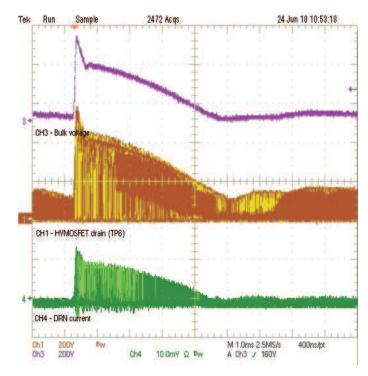
Figure 15. TRIAC Triggering at 50% (CH4 – 500 mA/10 mV)
