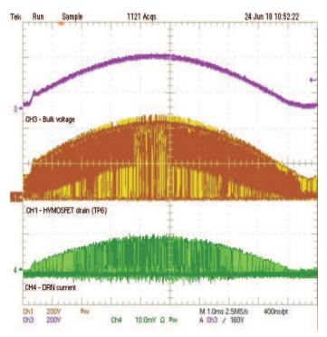
Figure 14. TRIAC Triggering at 100% (CH4 – 500 mA/10 mV)
