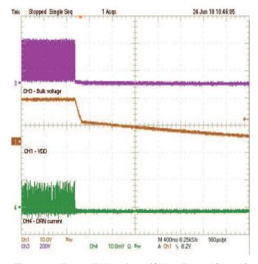
Figure 13. Turn-Off Waveform (CH4 - 500 mA/10 mV)
