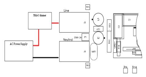
Figure 3. TRIAC Dimmer Test Setup
