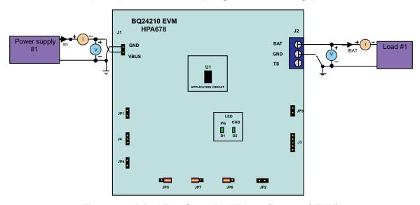
Figure 1. Original Test Setup for HPA678 (bq24210/2EVM)
