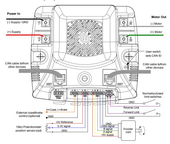
Figure 7-1. Advanced Wiring Diagram
