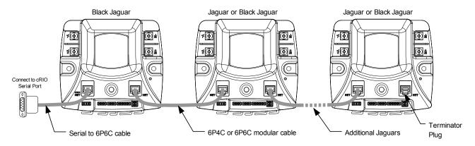
CAN cabling follows a daisy-chained topology using modular cable. Table 8-1 lists network parameters.
