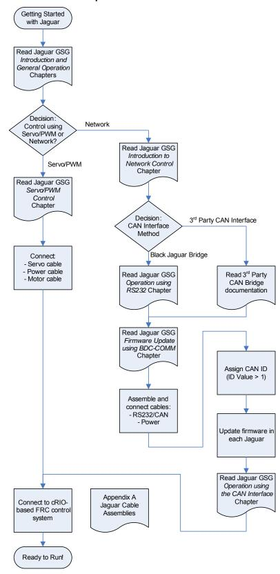
Figure 1-2. MDL-BDC24 Development Process
