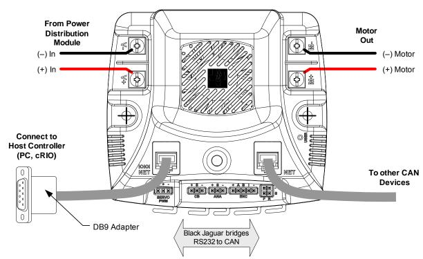
Figure 5-1. MDL-BDC24 Bridges for RS232 to CAN
