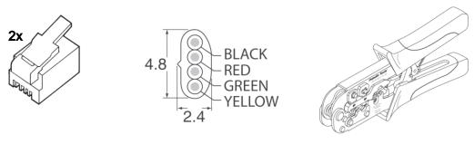
Modular plug for stranded flat oval cable AMP P/No. 5-641335 Digikey Stock No. A9092-ND Modular cable – 4 conductor Assmann Elect. AT-K-26-4-S/100-R Digikey Stock No. A0043R-100-ND
