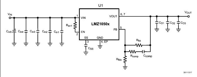
FIGURE 1. Component Schematic for Evaluation Board
