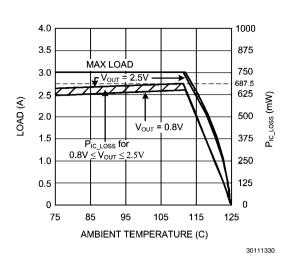
FIGURE 8. Current Derating vs. Ambient Temperature LMZ10503, V<sub>IN</sub> = 3.3V,  $\theta_{JA}$  = 20°C/W
