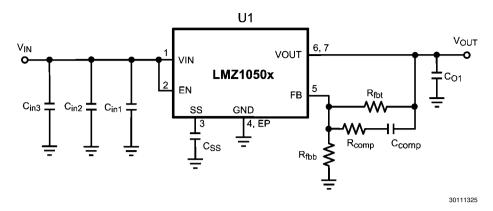
FIGURE 19. Component Schematic,  $V_{IN}$  = 5V,  $V_{OUT}$  = 2.5V, Complies with EN55022 Class B Radiated Emissions
