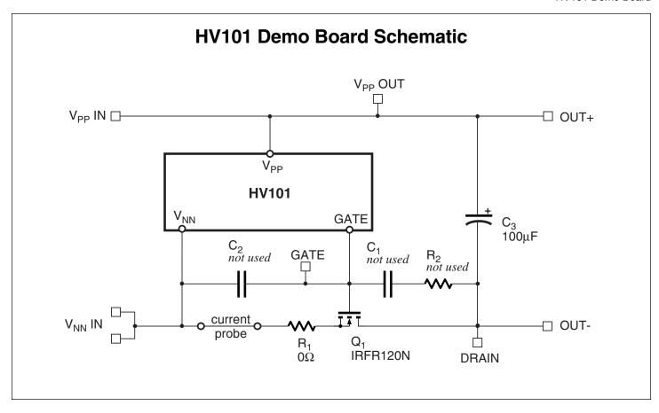
A very high dV/dt on the input can overload the HV101's internal gate clamp, causing turn-on transients. A capacitor in the  $\rm C_2$  position may be used to clamp the gate, preventing the transients. A 1nF value is usually adequate. Voltage rating should be 16 volts.
