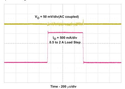
Figure 4. TPS54225EVM-538 Load Transient Response
