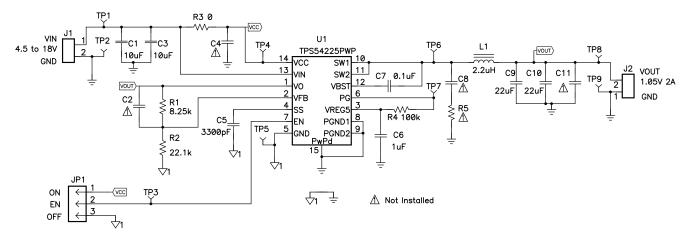
Figure 15. TPS54225EVM-538 Schematic Diagram
