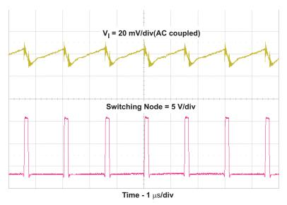
Figure 6. TPS54225EVM-538 Input Voltage Ripple
