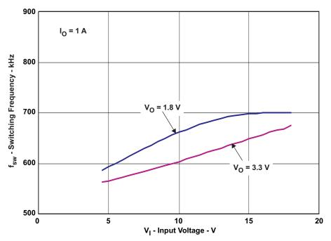
Figure 8. TPS54225EVM-538 Switching Frequency
