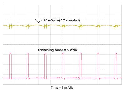
Figure 5. TPS54225EVM-538 Output Voltage Ripple
