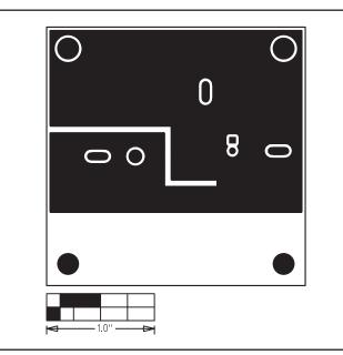
Figure 5. MAX5026 EV Kit PC Board Layout—Solder Side
