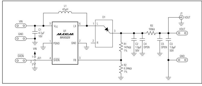
Figure 2. MAX5026 EV Kit Schematic
