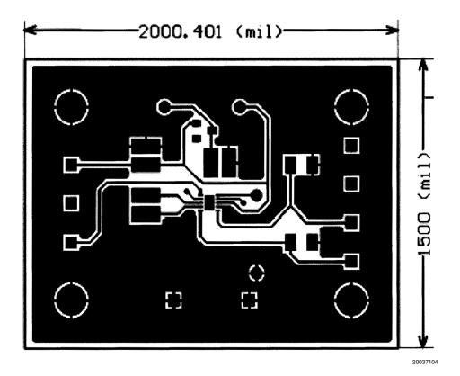
FIGURE 2. PCB Layout
