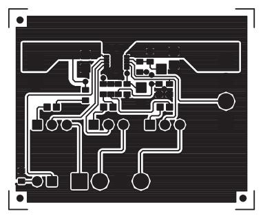
Figure 2. Board Layout Top Layer
