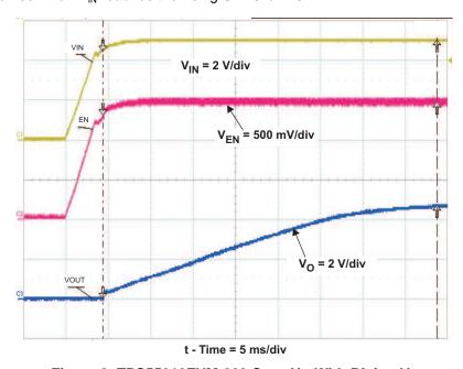
Figure 8. TPS55010EVM-009 Start-Up With Rising V<sub>IN</sub>
