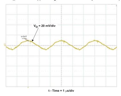
Figure 6. TPS55010EVM-009 Output Voltage Ripple
