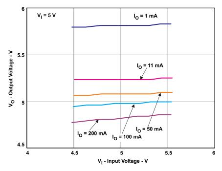
Figure 3. TPS55010EVM-009 Line Regulation, VIN = 5 V
