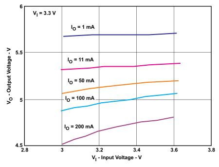
Figure 4. TPS55010EVM-009 Line Regulation, VIN = 3.3 V
