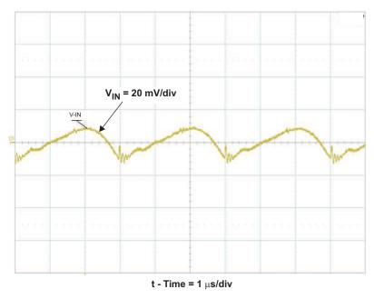
Figure 7. TPS55010EVM-009 Input Voltage Ripple
