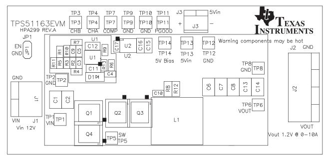
Figure 14. Top Layer Assembly Drawing (Top View)
