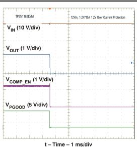
Figure 9. Output Overcurrent Protection
