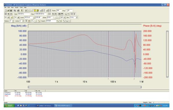
Figure 7. Loop Response Gain and Phase
