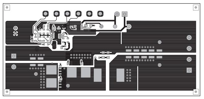
Figure 16. Top Copper (Top View)
