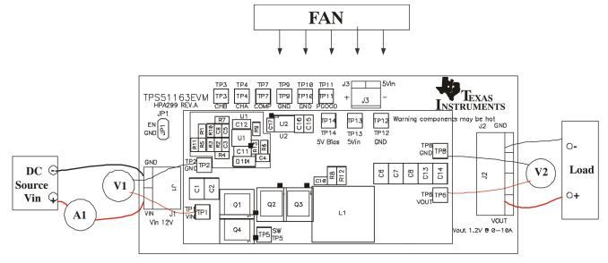
Figure 3. TPS51163EVM Recommended Test Set Up
