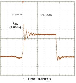
Figure 11. Switch Node Waveform
