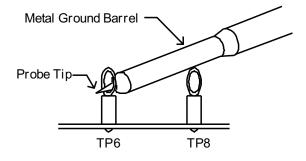
Figure 2. Tip and Barrel Measurement for V<sub>OUT</sub> Ripple
