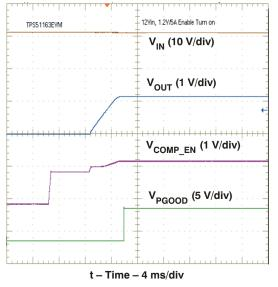
Figure 12. Enable Turn-On
