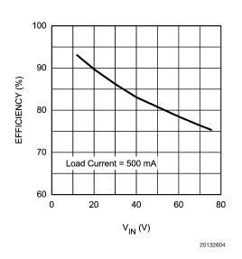
FIGURE 3. Efficiency vs V<sub>IN</sub>
