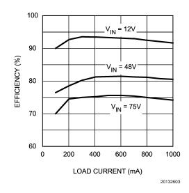
FIGURE 2. Efficiency vs Load Current
