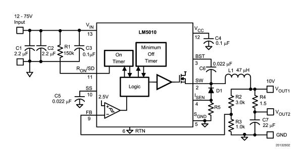
FIGURE 4. Board Schematic
