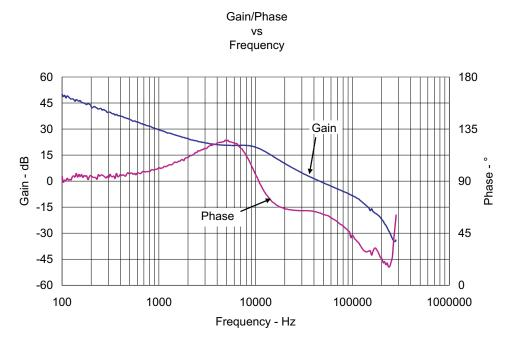
Figure 12. TPS40195EVM Bode Plot  $V_{IN}$  = 12 V,  $I_{OUT}$  = 0 A, Crossover Frequency = 46 kHz, Phase Margin = 62°
