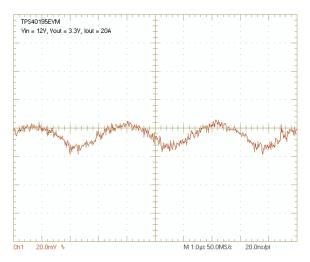
Figure 8. TPS40195EVM Output Voltage Ripple ( $V_{IN}$  = 12 V,  $I_{OUT}$  = 20 A)
