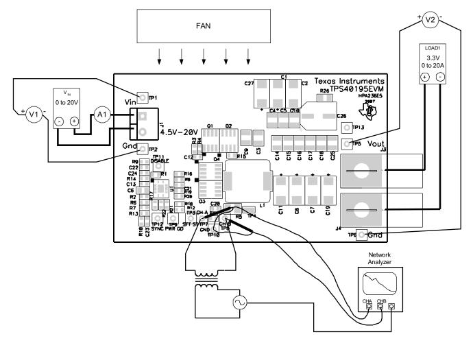
Figure 4. Control Loop Measurement Setup
