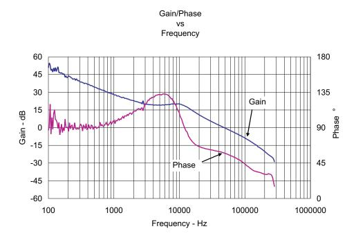
Figure 11. TPS40195EVM Bode Plot  $V_{IN}$  = 12 V,  $I_{OUT}$  = 20 A, Crossover Frequency = 48 kHz, Phase Margin = 57.5°
