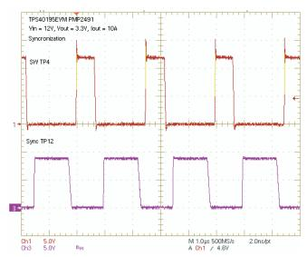
Figure 15. TPS40195EVM Switching Waveform (Ch1: TP4) and Synchronization (Ch2: TP12)  $V_{\text{IN}} = 12 \text{ V}$ ,  $I_{\text{OUT}} = 10 \text{ A}$ ,  $f_{\text{SYNC}} = 400 \text{ kHz}$
