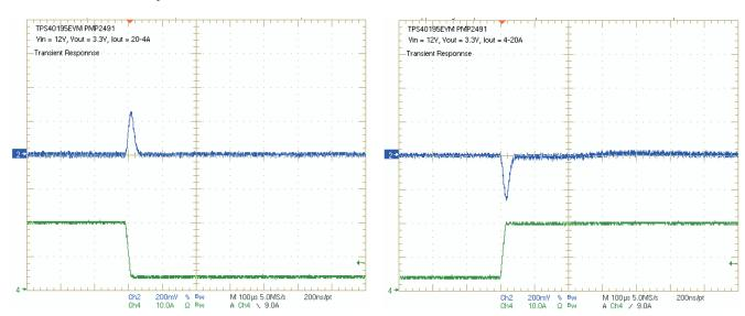
Figure 9. TPS40195EVM Transient Response,  $V_{IN}$  = 12 V,  $I_{OUT}$  = 20 A to 4 A, Ch1:  $I_{OUT}$ , Ch2:  $V_{OUT}$
