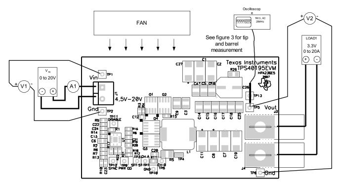
Figure 2. TPS40195EVM Recommended Test Set-Up
