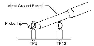
Figure 3. Output Ripple Measurement - Tip and Barrel Using TP5 and TP13
