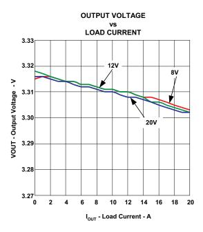
Figure 6. TPS40195EVM Line and Load Regulation  $\rm V_{IN}$  = 8 V to 20 V,  $\rm V_{OUT}$  = 3.3 V  $\rm I_{OUT}$  = 0 A to 20 A
