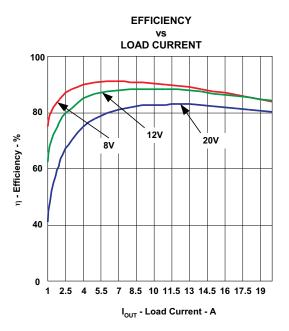
Figure 7. TPS40195EVM Efficiency  $\rm V_{IN}$  = 8 V to 20 V,  $\rm V_{OUT}$  = 3.3 V  $\rm I_{OUT}$  = 1 A to 20 A
