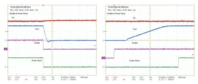
Figure 13. TPS40195EVM Disable and Power Good,  $V_{IN}$  = 12 V,  $I_{OUT}$  = 10 A, Ch1: TP1 ( $V_{IN}$ ), Ch2: TP5 ( $V_{OUT}$ ), Ch3: TP11 (ENABLE); Ch4: TP9 (Power Good)
