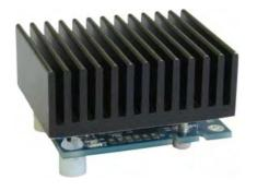
TE-CORE thermoharvesting power module with integrated TGP offers an efficient DC-booster and power management concept.
