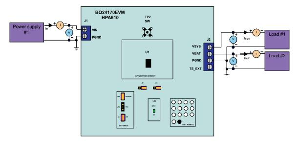
Figure 1. Original Test Setup for HPA610A (bq24710EVM)
