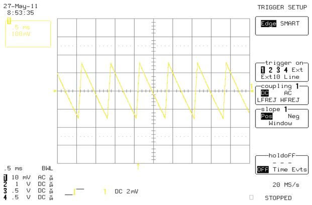
Figure 2. Boost Output Ripple : Vbat = 3.2 V and 1 mA Load on Boost
