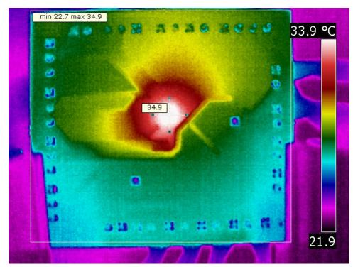
Figure 17. Thermal Performance – Bottom Side
