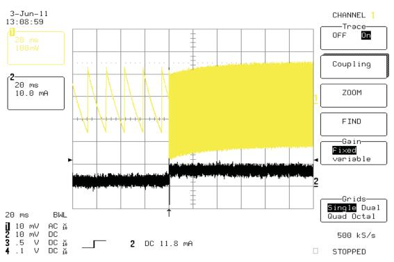
Figure 9. Load Transient, Boost : Vbat = 3.6 V with 0 mA to 5 mA Transient, Constant 15 mA Load on LDO. CH3 Bstout CH4 IBOOST
