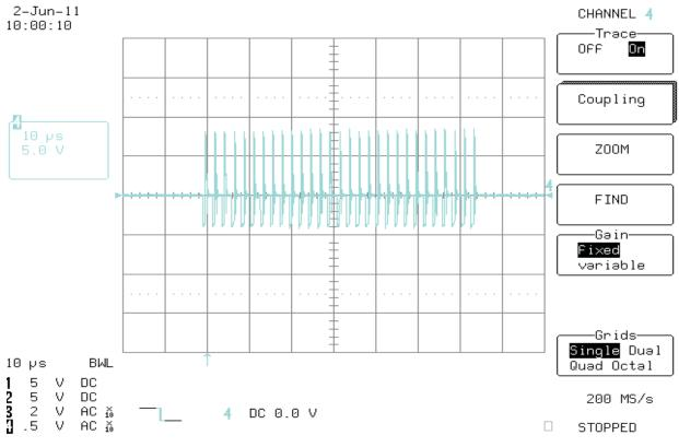
Figure 8. Switchnode : Vbat = 3.6 V, No Load, 10 µs/div
