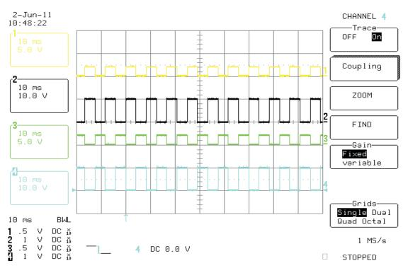
Figure 13. H-Bridge Operation : Ch. 1 - Function Generator Input to HBR1, Ch. 2 - LCRP output, Ch. 3 - Function Generator Input to HBR2, Ch. 4 - LCRN output
