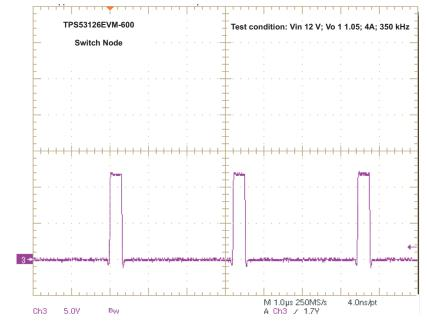
Figure 10. Switching Waveform ( $V_{IN}$  = 12 V,  $V_{OUT1}$  = 1.05 V,  $I_{OUT1}$  = 4 A,  $F_{SW}$  = 350 kHz)
