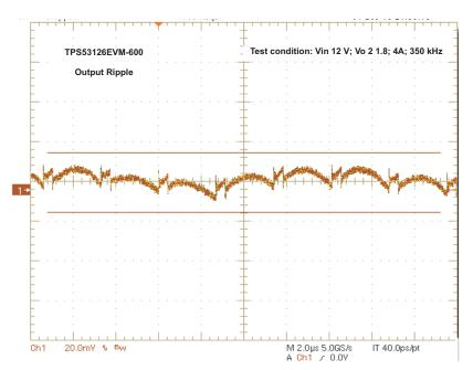
Figure 9. Output Voltage Ripple ( $V_{IN}$  = 12 V,  $V_{OUT2}$  = 1.8 V,  $I_{OUT2}$  = 4 A,  $F_{SW}$  = 350 kHz)
