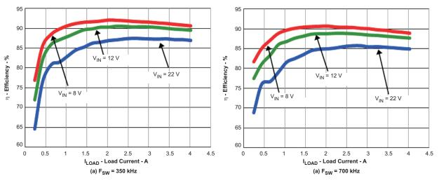
Figure 5. Efficiency vs Load (V<sub>IN</sub> = 8 V–22 V, V<sub>OUT2</sub> = 1.8 V, I<sub>OUT2</sub> = 0 A–4 A)
