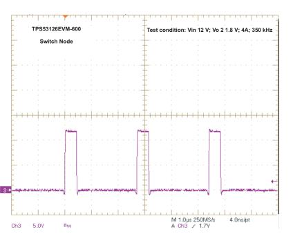
Figure 11. Switching Waveform ( $V_{IN}$  = 12 V,  $V_{OUT2}$  = 1.08 V,  $I_{OUT2}$  = 4 A,  $F_{SW}$  = 350 kHz)
