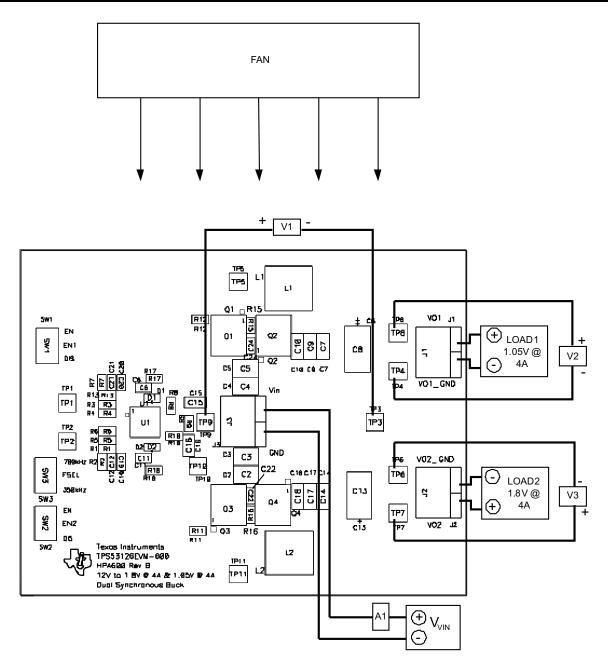
Figure 3. TPS53126EVM-600 Recommended Test Setup
