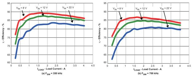
Figure 4. Efficiency vs Load ( $V_{IN}$  = 8 V–22 V,  $V_{OUT1}$  = 1.05 V,  $I_{OUT1}$  = 0 A–4 A)
