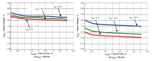
Figure 7. Output Voltage vs Load ( $V_{IN} = 8 V-22 V$ ,  $V_{OUT2} = 1.8 V$ ,  $I_{OUT2} = 0 A-4 A$ )
