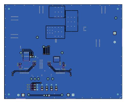
Figure 10. Bottom Assembly Layer
