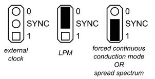
Figure 5. SYNC Jumper Setting
