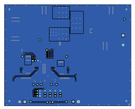
Figure 11. Bottom Layer Routing
