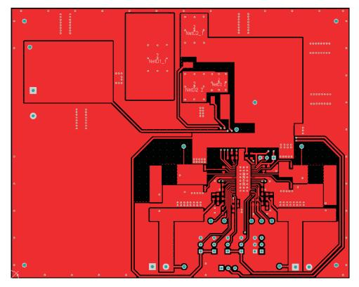
Figure 9. Top Layer Routing
