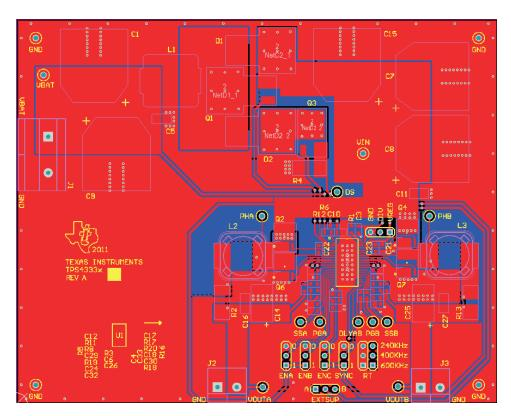
Figure 8. Top Assembly Layer
