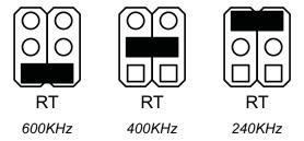
Figure 6. RT Jumper Setting
