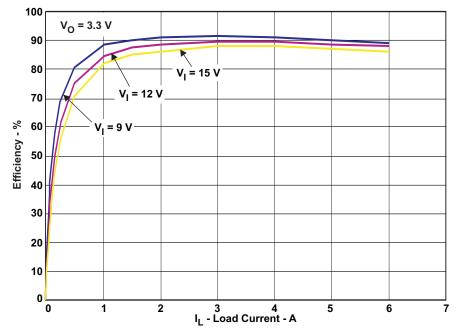
Figure 2. Efficiency vs Voltage at 25°C
