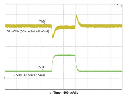
Figure 8. 3.3-V TPS84620EVM-692 Transient Response at 25°C
