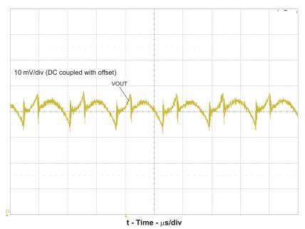
Figure 10. TPS84620EVM-692 Output Voltage Ripple
