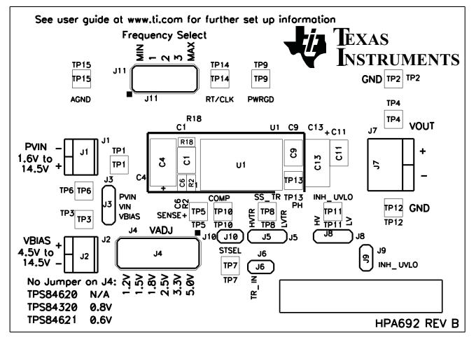
Figure 13. TPS84x2xEVM-692 Top-Side Layer and Assembly
