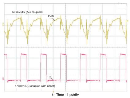
Figure 11. TPS84620EVM-692 Input Voltage Ripple
