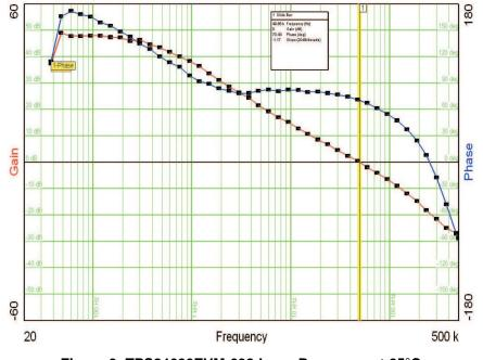
Figure 9. TPS84620EVM-692 Loop Response at 25°C
