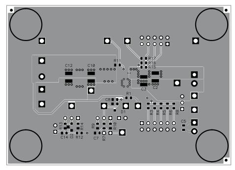
Figure 16. TPS84x2xEVM-692 Bottom-Side Layer and Assembly
