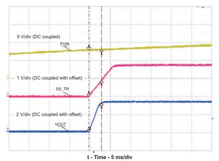
Figure 12. TPS84620EVM-692 Start-Up Waveforms With Rising PVIN
