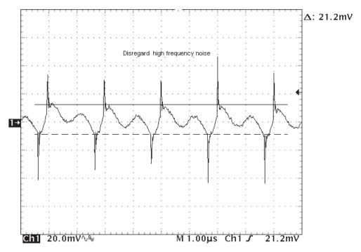
Figure 13. VOUT2 Output Ripple, (VIN = 12 V,  $I_{OUT2}$  = 10 A)
