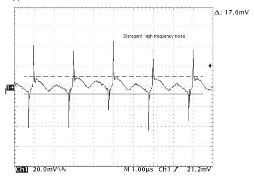
Figure 12. VOUT1 Output Ripple, (VIN = 12 V,  $I_{OUT1}$  = 10 A)
