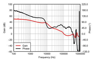
Figure 10. TPS40322EVM-679 VOUT1 Loop Response Gain and Phase, (VIN = 12 V I<sub>OUT1</sub> = 10 A)
