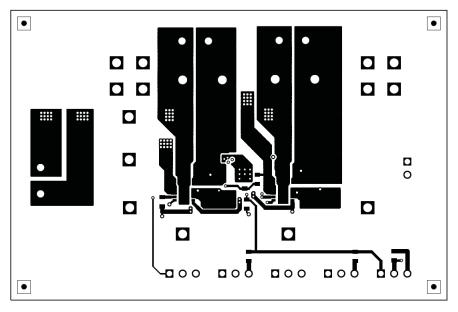
Figure 21. Top Copper (top view)
