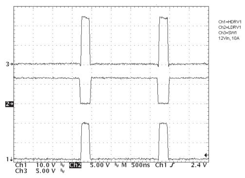
Figure 14. Output 1 Switching waveform, (Ch1 = HDRV1, Ch2 = LDRV1, Ch3 = SW1, VIN = 12 V,  $I_{OUT1}$  = 10 A)
