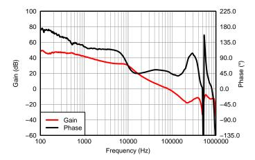
Figure 11. TPS40322EVM-679 VOUT2 Loop Response Gain and Phase, (VIN = 12 V  $I_{OUT2}$  = 10 A)
