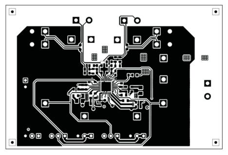
Figure 22. Bottom Copper (bottom view)
