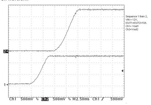
Figure 15. Enable Turn-On Waveform, (Sequencing VOUT1 then VOUT2, Ch1 = VOUT1, Ch2 = VOUT2, VIN = 12 V,  $I_{OUT1} = I_{OUT2} = 10$  A)
