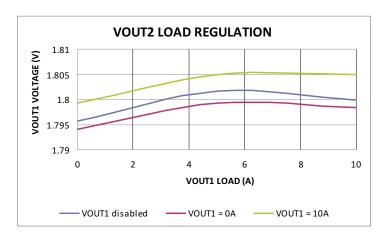
Figure 7. TPS40322EVM-679 VOUT2 Load Regulation, (VIN = 12 V)
