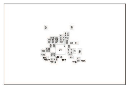
Figure 20. Bottom Assembly Drawing (bottom view)
