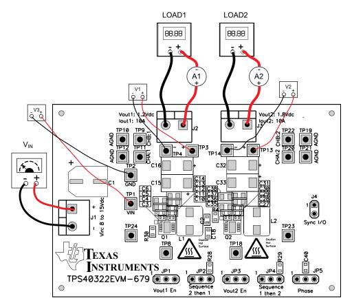
Figure 2. TPS40322EVM-679 Recommended Test Set Up
