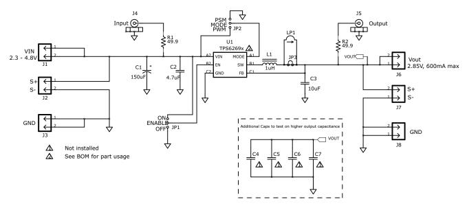
Figure 1. TPS6269xEVM Schematic
