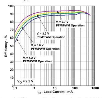
Figure 4. Efficiency vs Load current for the TPS62691
