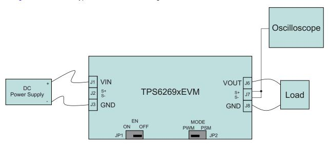
Figure 3. Hardware Board Connection
