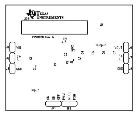
Figure 10. TPS62690/1/2/3EVM Component Placement (Top View)
