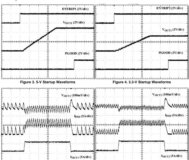
Figure 5. 5-V Load Transient Response
