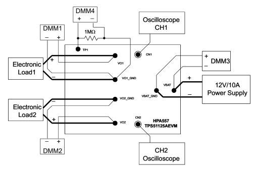
Figure 2. Equipment Setup for TPS51125AEVM board
