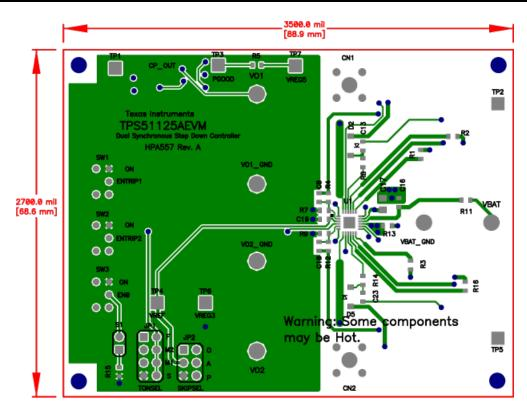
Figure 7. Top Layer Routing
